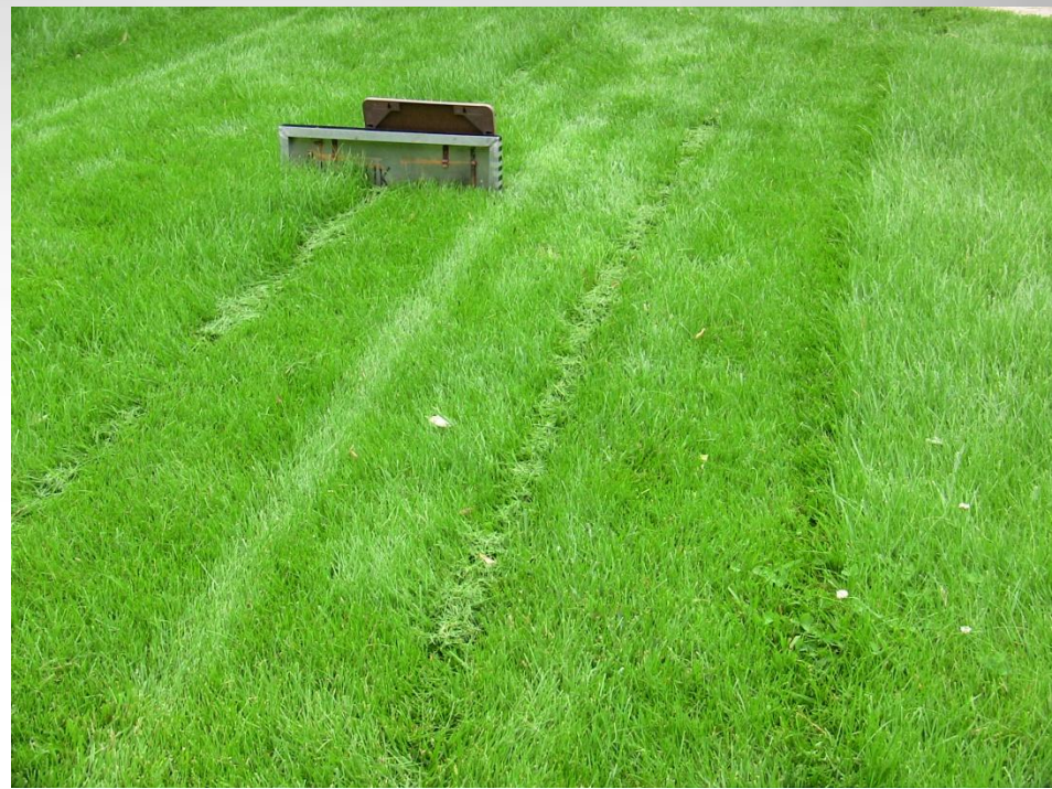
Competitor A overall view from opposite direction, significant grass accumulated in wheel tracks
