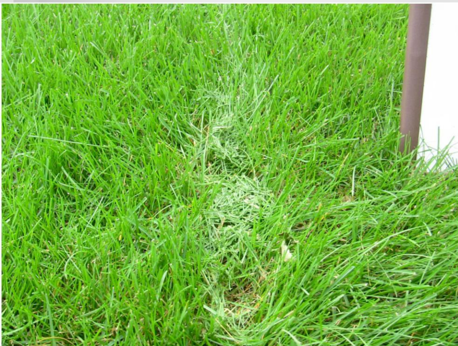
Toro blade minor dribbling of grass along wheel tracks
